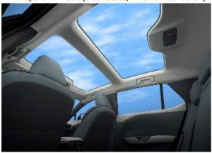
Once arranged into a random pattern, the special material diffuses light from the outside to turn the glass opaque and reduce glare.
