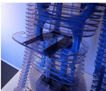
THK's FBL27D slide rails are used in the ATMOS II's chest to allow a microcomputer to be installed. THK's RF77F cross-roller ring is also used in the waist.
