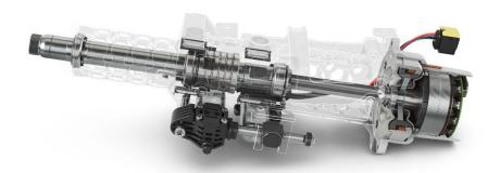
The adjustable Hand Wheel Actuator transmits the steering angle via the vehicle electronics to the steering gear, while the Force Feedback Actuator generates the specific steering feel. Photo: Schaeffler
